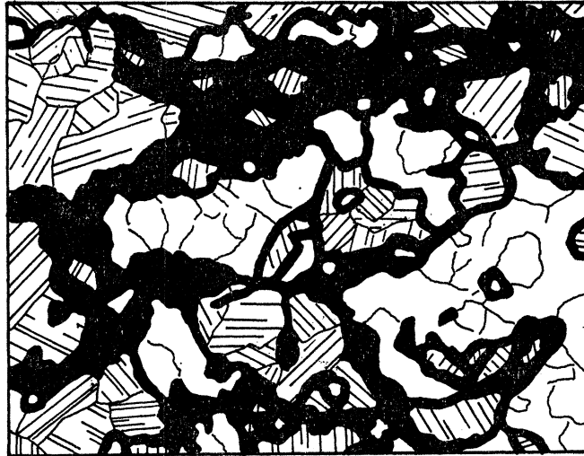
FIGURE 1. Partially melted granite gneiss block, Grube Mertens, Gemündener Maar, Westeifel (see Frechen 1971). Ornaments: black, glass + vesicles; lined ornament, feldspar (mainly plagioclase); no ornament, quartz (grain boundaries indicated). Larger areas of glass are brown and contain opaque mineral aggregates after biotite. Narrower veins of glass on quartz–feldspar boundaries are colourless. The development of the melt along feldspar–quartz boundaries and around biotite grains is a striking feature of the specimen. Modal analysis gives glass, 35%; vesicles, 10%; feldspar + quartz, 55%. Field of view is 5 \times 4 mm.
